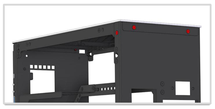
**REASSEMBLY NOTE:** When putting the top panel back on the case it is recommended to position the tabs on the rear corners first, then place the rear flange onto the outside of the frame. This will position the front flange correctly.
