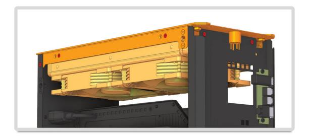
Make sure rear flange is on the outside of the rear chassis. There are 4x M3 x 5mm FLAT HEAD screws.
