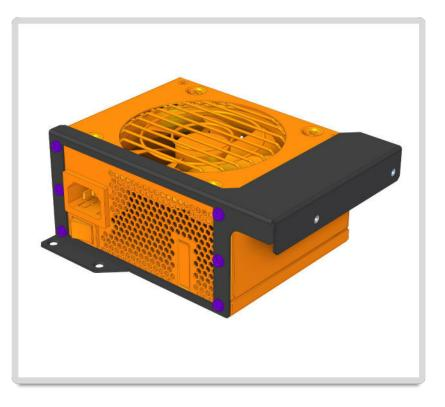
Once the SFX PSU is attached to its mounting bracket and the cables are routed into position, the SFX PSU can be screwed back in via the **4x M3x5mm FLAT HEAD** screws removed in the last step.
