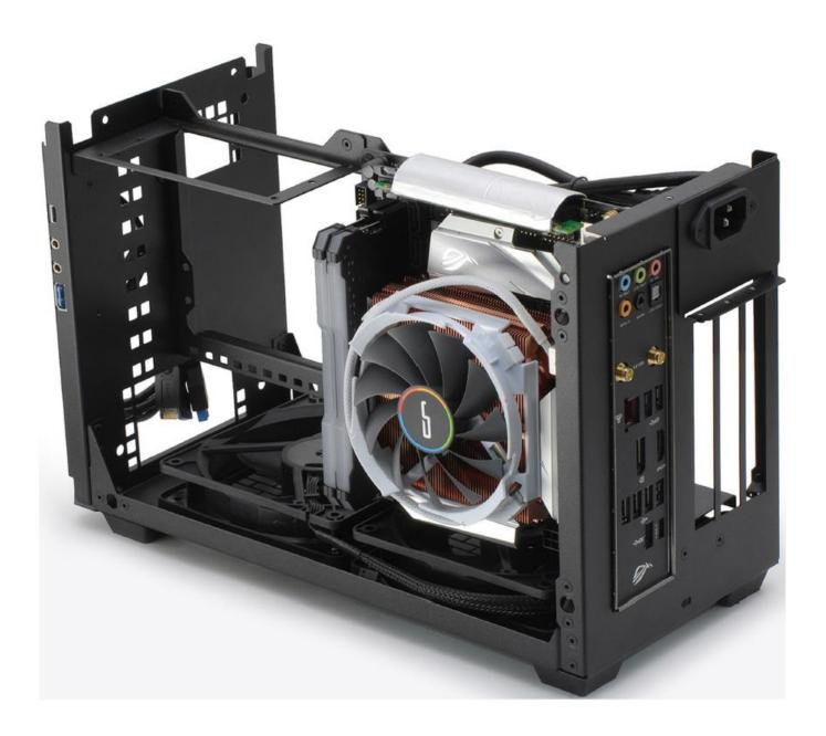
It is recommended to install your CPU, RAM, and CPU cooler onto your motherboard before placing the motherboard into the case. This is recommended because some CPU coolers are not easy to install, which is further complicated by the riser and middle rib inside the case. The motherboard is mounted with **Type 3-M3.5 TRUSS HEAD** screws.
