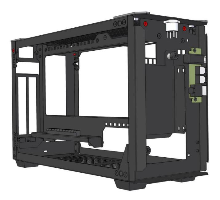
The top panel on the SM550 / SM560 is held on via **Type 2 M3 flat** head screws, each with a Phillips #1 head.
