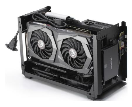
PCIe cards are secured with up to 3x Type 1 M3x6 PAN HEAD.
