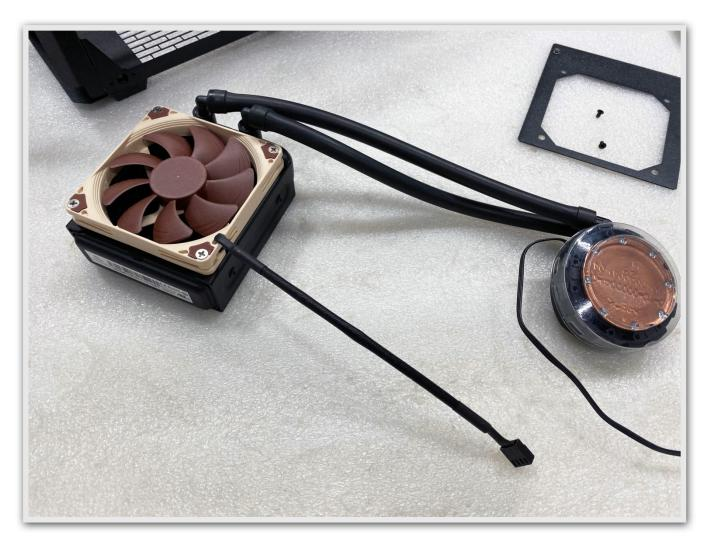
**NOTE: Sliger** does **NOT** include the crews for attaching the fan to the radiator. We recommend 4x .750" long 6-32 Phillips #2 flat head screws.
